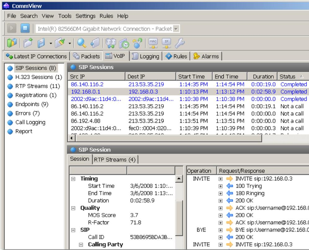
Using CommView, you can analyze signaling sessions and RTP streams in real time, watch the charts and diagrams to understand the quality problems that may affect your VoIP network (packet loss, jitter, or sequence errors), monitor MoS and R-factor for every call, and even listed to the actual calls. Yes, CommView can record and play back them for you.
