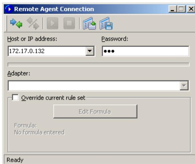
Click on the **New Remote Agent Connection** button to establish a new connection, or click on the **Load Remote Agent Profile** toolbar button to load a previously saved Remote Agent connection profile. A previously saved profile may also be loaded from the New Remote Agent Connection window.
