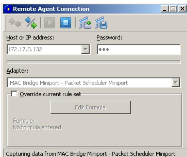
CommView will start to capture the remote computer's traffic as if it's your local network traffic; there is virtually no difference between using CommView locally and remotely. When you are done with remote monitoring, just click on the **Stop Capture** toolbar button. You can then change the adapter or disconnect from Remote Agent by clicking the **Disconnect** toolbar button. To return to the standard mode, click **File => Remote Monitoring Mode**, and the additional toolbar will disappear.
