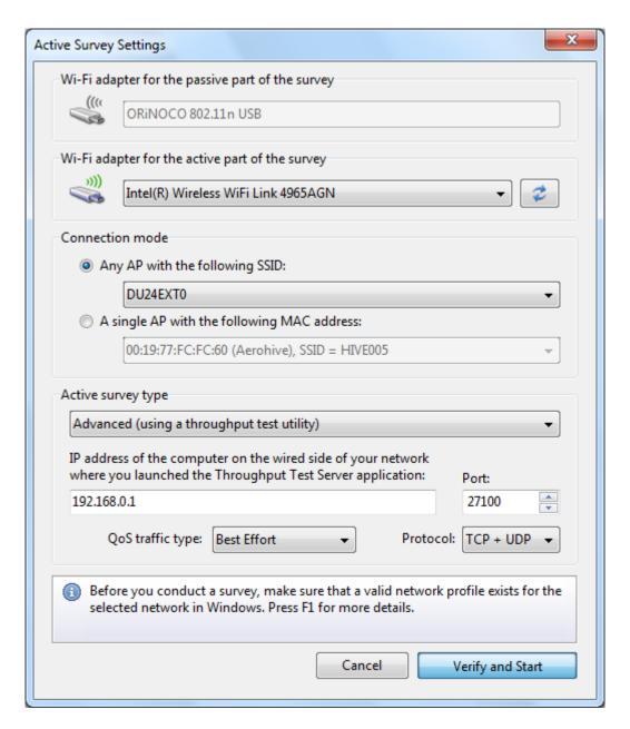
This dialog allows you to configure TamoGraph for an active survey you are about to conduct.
