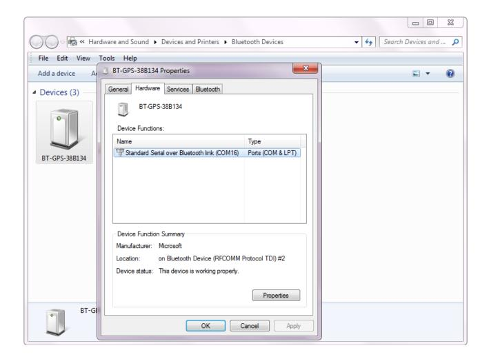
For USB devices, open **Device Manager** and find your device under **Ports (COM & LPT)**. The device name will be followed by the port number, as shown below.
