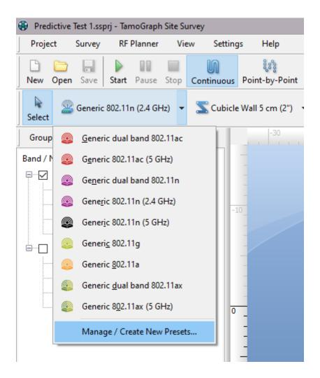
This opens the **Preset Manager** where you can modify all the AP parameters and change the antenna type. The screenshot below illustrates a few changes we made to the default values for the 5 GHz radio to ensure that the virtual AP matches the real-world Aruba AP-325 APs that we will deploy:
