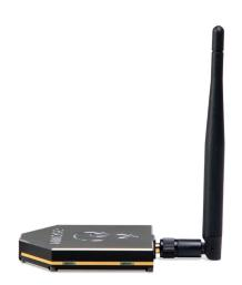
When a dual-band model, Wi-Spy DBx, is used, it continuously sweeps both bands, one after the other. Using two Wi-Spy DBx units simultaneously might improve data quality, as TamoGraph would dedicate each of the units to one band only. Note that you cannot use two WiPry devices of the same type simultaneously. You can, however, combine WiPry Clarity and WiPry 2500x, and you can mix Wi-Spy and WiPry devices.
