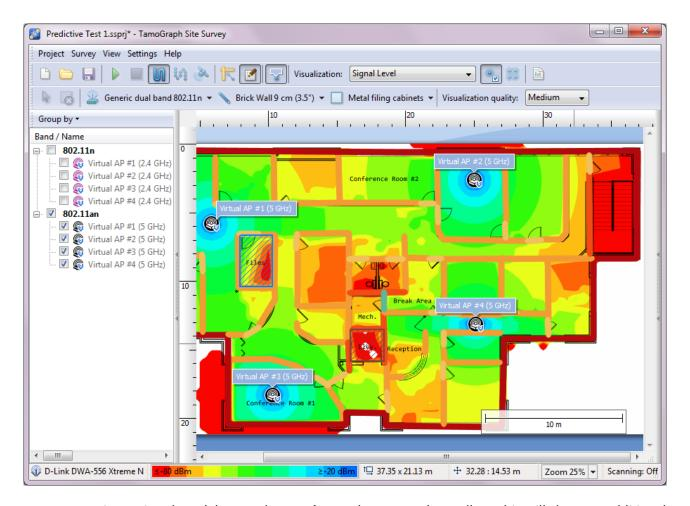
To start creating a virtual model, press the **RF Planner** button on the toolbar. This will show an additional toolbar with a few drawing tools. It is recommended to begin by drawing walls. Once the walls have been drawn, you can place APs on the floor plan, decide how many APs you need to provide adequate coverage, select the best positions for the APs, and configure their parameters (channel numbers, rates, antennas, etc.)
