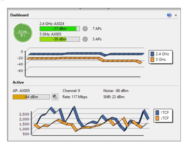
If TamoGraph detects a Wi-Fi adapter that can be used for **passive surveys**, the dashboard includes the following indicators:
