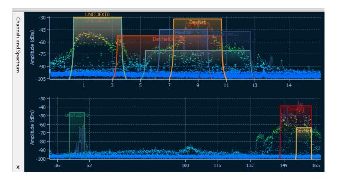
When a USB spectrum analyzer is plugged in, a live spectrum picture is displayed on the **Channels and Spectrum** pane of the main CommView for WiFi window, as shown below.
